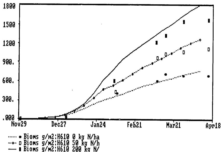
**Multiple-treatment, single-variable plot.** The second graph was generated after running the CERES MAIZE model for three treatments or runs (variety H610 with 200, 50, and 0 kg N/ha). In the example shown, only one variable (biomass) is plotted for each of the runs.
